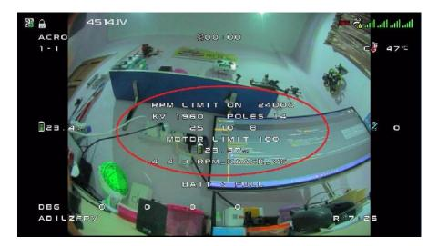
f. Race Director/ Race Controller will use the active "Debug RPM Limit" reading from the drone OSD to check compliance to the 24,000 RPM Limit during the race. During race, motor RPM should not exceed 26,000 as indicated in the "Debug" OSD. Race Director has the right to disqualify pilot if drone is shown of not complying to this requirement.
